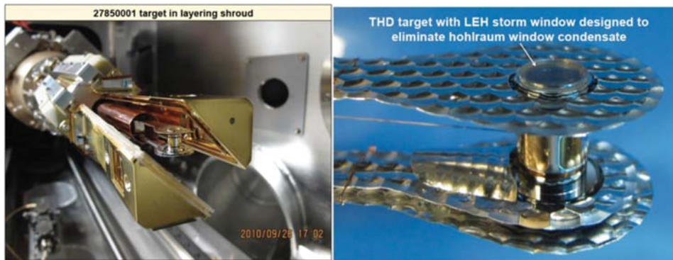
FIG. 100. (a) Cryo-layered target in its protective shroud. (b) Cryo-layered target showing the LEH storm window developed in 2010–11 to protect the hohlraum windows from condensation of residual chamber gas.
